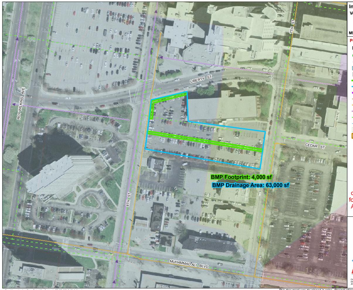
**Ohio River Sewershed** Solution ID # L\_OR\_MF\_053\_S\_12\_A\_A MSD Main Office Parking Lot Biofiltration Swale
