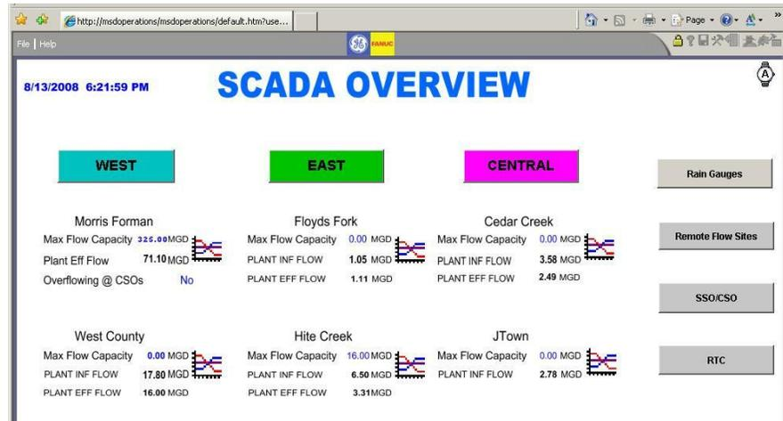
MSD's SCADA system is connected to the Plant Information System (PI) and iHistorian databases. These two systems pull data from the SCADA system and store the data from the date the attribute tag is created until the attribute tag is disabled.
