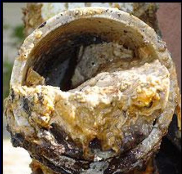
Grease accumulates in pipes
