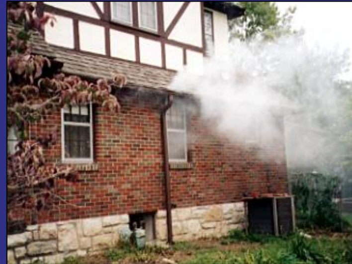
Smoke testing on public sewer indicates improper downspout connection to the sanitary sewer
