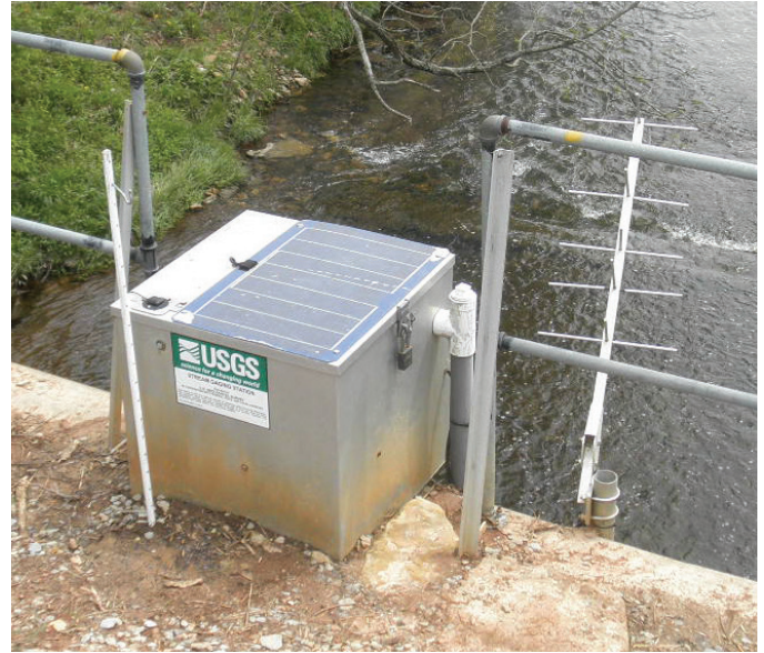
This USGS streamflow gage (gray box in photo) is located on Cedar Creek at Thixton Lane. This type of gage is used to continuously monitor stream temperature, dissolved oxygen, and stream flow. The antenna to the right of the box transmits data to a satellite for real time monitoring results via the web at http://waterwatch.usgs.gov
