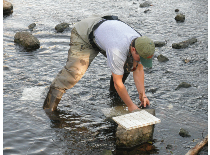
Placing ceramic tiles for collecting algae in the Middle Fork of Beargrass Creek.
