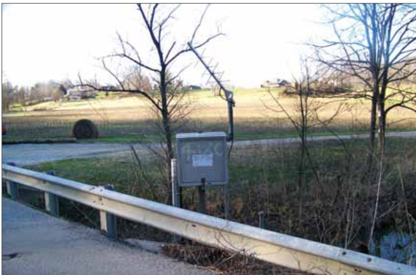
This USGS flow gage (gray box) is located on Brier Creek at Bear Camp Road. The gage is used to continuously monitor dissolved oxygen and stream flow. The antenna on top transmits data for real time monitoring results.
