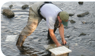
Placing ceramic tiles for collecting algae in the Middle Fork of Beargrass Creek.
