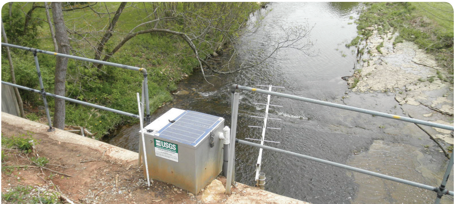
This USGS streamflow gage (gray box in photo) is located on Cedar Creek at Thixton Lane. This type of gage is used to continuously monitor stream temperature, dissolved oxygen, and stream flow. The antenna to the right of the box transmits data to a satellite for real time monitoring results via the web at http://waterwatch.usgs.gov
