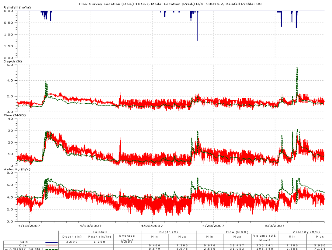
FIGURE 2.4.31 EXAMPLE CALIBRATION/VALIDATION HYDROGRAPH CARDINAL SEWER - UNION AND FAYETTE AVENUE
