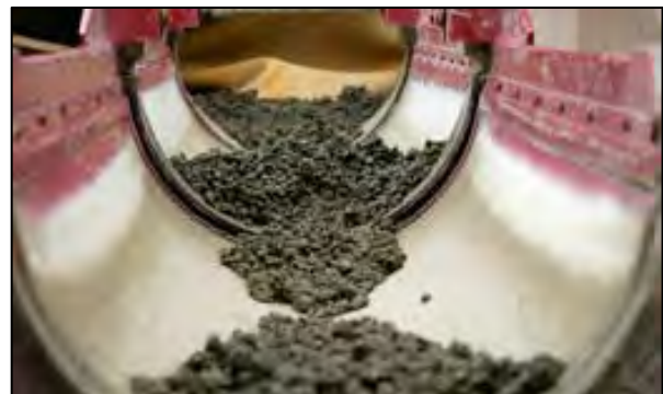
Pervious concrete contains less lime and finer particles than ordinary concrete.
