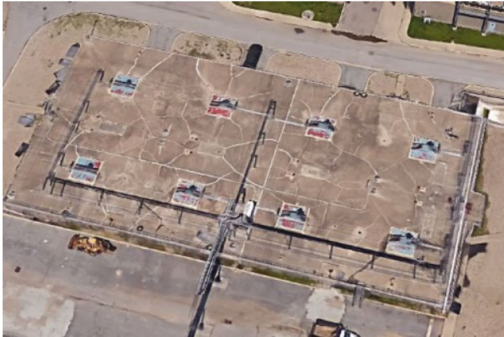
HPO Reactor "A" Filled cracks (Photo: Google Earth)
