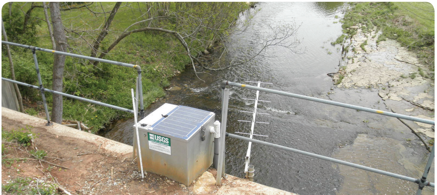
This USGS streamflow gage (gray box in photo) is located on Cedar Creek at Thixton Lane. This type of gage is used to continuously monitor stream temperature, dissolved oxygen, and stream flow. The antenna on top of the box transmits data to a satellite for real time monitoring results via the web at http://waterwatch.usgs.gov
